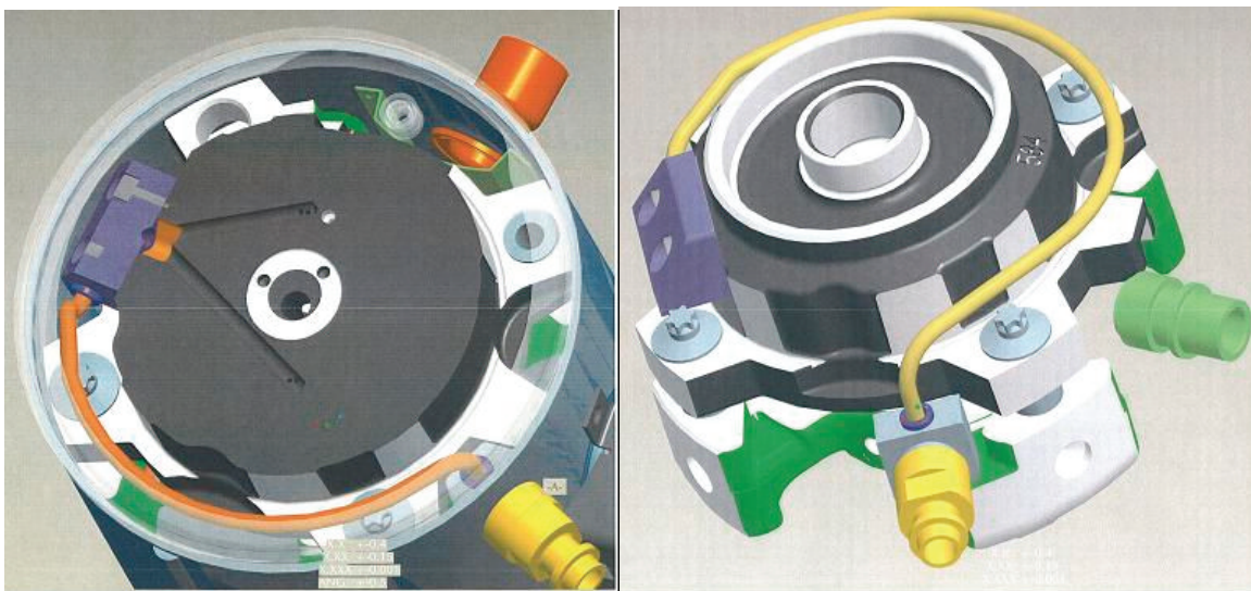
Figure 5. Injection Tube in ZH-KVE Compressor and Scroll Injection Ports
